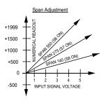
signal change. The input summing resistor values are weighted in a binary progression, so they can be switched in combinations to give 32 discrete steps of span. The fine adjust control brackets these coarse steps and can be adjusted to the exact span needed.
