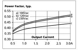
Nov. 2020 / Rev. 2.2 DS-ML15.051-EN All parameters are specified at 5V, 3A, 230Vac input, 25°C ambient and after a 5 minutes run-in time unless otherwise noted.
