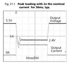
Peak load 6A (resistive load) for 50ms Output voltage dips from 5.1V to 2.4V.
