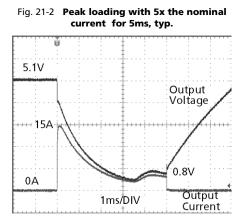
Peak load 15A (resistive load) for 5ms Output voltage dips from 5.1V to 0.8V.
