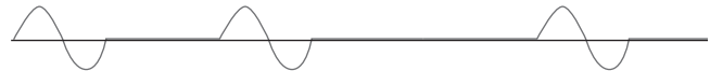
Figure 5.2b — 40% single cycle variable time base 1 cycle on, 1 cycle off, 1 cycle on, 2 cycles off.
