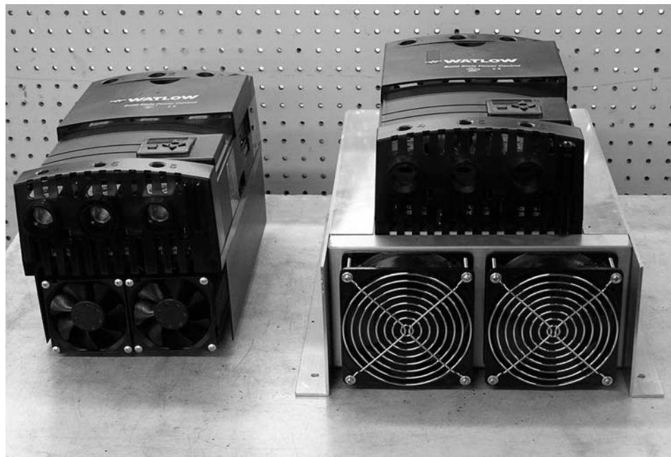
Figure 2.4 — The F35 Power Series (right) is cooled with larger fans.
