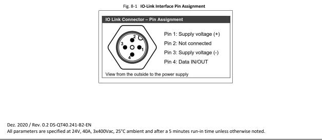
In order to operate the IO-Link interface it is required to install/upload the IODD-File (IO-Link Device Description) into the connected IO-Link master in the first step. The most recent IODD File can be found on the PULS website (<u>www.pulspower.com</u>) in the product download section of the product page of QT40.241-B2. The device can be accessed via IO-Link also, if the power supply is not connected to AC-mains and switched off.
