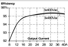
Fig. 11-1 Efficiency vs. output current at 24V, typ.
