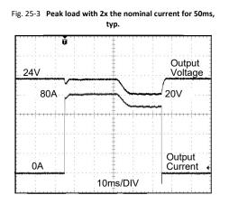
80A Peak load (resistive) for 50ms Output voltage dips from 24V to 20V.
