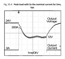
200A Peak load (resistive) for 5ms Output voltage dips from 24V to 12V.
