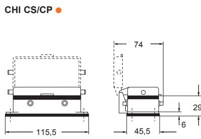
**Q** **IMPORTANT NOTE:** The enclosures ensure IP66/IP69 degree of protection (or IP65 for hinged cover versions) when mated and locked with the closing levers. The cover (CS, CP) only ensures mechanical protection, but does not ensure IP65 degree of protection.
