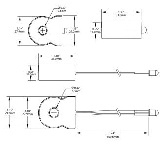
Note: Panel opening should be 0.267 to 0.273", panel thickness 0.32 to 0.125"
