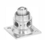
125B 125B-3-10-21 Model 125B is a 0.125-inch orifice, ball-operated valve that can be actuated from any angle. Its hardened steel ball is captive and free turning. The valve's short-stroke actuation is fully open at 0.031-inch; maximum stroke is 0.062-inch. The 125B can be mounted in-line, on mounting base, with panel mounting nuts, or with body threads.
