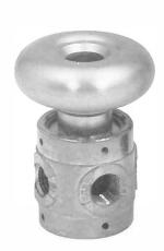
250HO 250HO-3-10-20 Model 250HO is a 0.250-inch orifice, normally closed, detented, palm-operated valve. Detent is achieved by pressing the large aluminum palm actuator; valve is returned to the normally closed position by pressing the red center-button. The 250HO functions as a pneumatic "circuit breaker" and automatically closes if there is a sudden loss of pressure (below approximately 12 psig); valve must be manually reopened. The pressure range of the 250HO valve is 25-125 psig.
