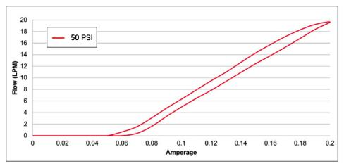
Calibrated with stabilized upstream pressure of 50 PSI to a flow of 18 SLPM @ 200mA.
