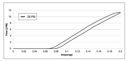
PV3PM1203250 will have precision control but less flow when upstream pressure is lower than 50 PSI. Typical curve with stabilized upstream pressures of 25 PSI is shown.
