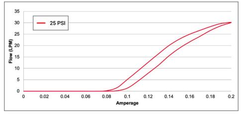
Calibrated with stabilized upstream pressure of 25 PSI to a flow of 30 SLPM @ 200mA. PV10PM2408025 will have precision control but less flow when the stabilzed upstream pressure is lower than 25 PSI.
