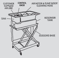
The portable clutch & brake cleaning system consists of a reservoir tank, a cleaning sink and cover/tray, a hose with a cleaning attachment, and a scissors base. The auto service technician raises the scissors base to bring the sink up to the brake or clutch assembly, then turns on the motor and begins cleaning.
