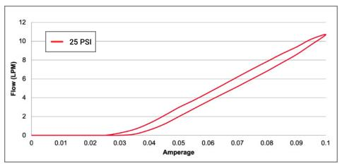
Calibrated with stabilized upstream pressure of 25 PSI to a flow of 10 SLPM @ 100mA. PV3EP2403225 valve will have precision control but less flow when the stabilized upstream pressure is lower than 25 PSI.
