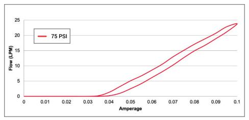
Calibrated with stabilized upstream pressure of 75 PSI to a flow of 25 SLPM @ 100mA.
