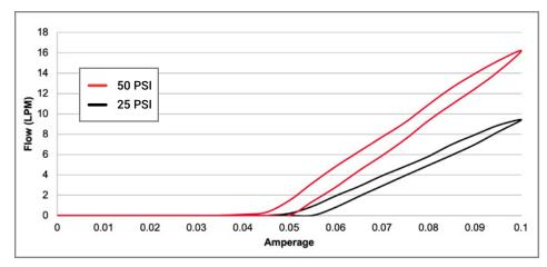
PV3PM2403275 will have precision control but less flow when upstream pressure is lower than 75 PSI. Typical curves with stabilized upstream pressures of 25 and 50 PSI are shown.
