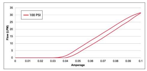
Calibrated with stabilized upstream pressure of 100 PSI to a flow of 30 SLPM @ 100mA.
