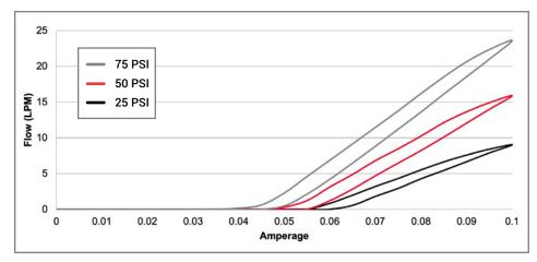
PV3P24032A0 will have precision control but less flow when upstream pressure is lower than 100 PSI. Typical curves with stabilized upstream pressures of 25, 50 and 75 PSI are shown.
