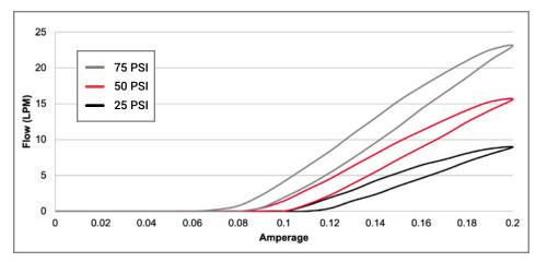
PV3PM12032A0 will have precision control but less flow when upstream pressure is lower than 100 PSI. Typical curves with stabilized upstream pressures of 25, 50 and 75 PSI are shown.
