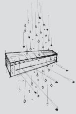
Humphrey developed a special valve manifold assembly with nozzles spaced 0.120 inches apart for a customer who was building a system to separate recycled multicolored glass particles by using jets of air.
