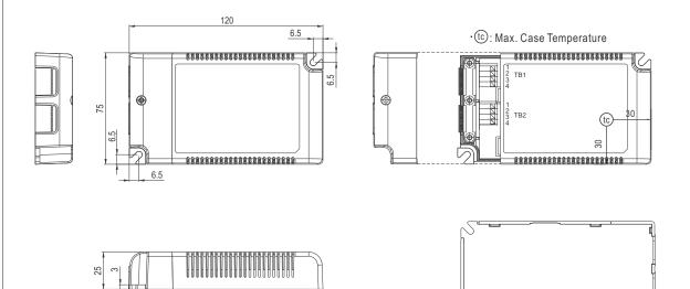
NOTE: Please use wires with a cross section of  $0.75 \sim 1.5 \text{mm}^2$  for TB1 and wires with a cross section of  $0.5 \sim 1.5 \text{mm}^2$  for TB2.
