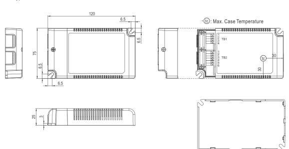
NOTE: Please use wires with a cross section of 0.75~1.5mm² for TB1 and wires with a cross section of 0.5~1.5mm² for TB2.
