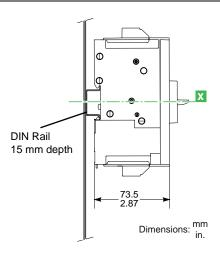
Dimensions 15 to 125 A Circuit Breakers
