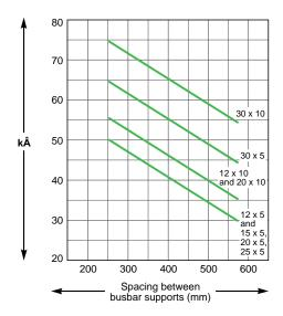
Short-circuit strength diagram according to UL845 (LA9ZX01508).
