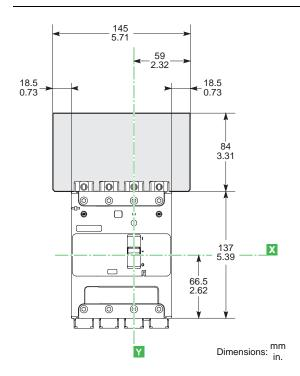
Dimensions 15 to 125 A Circuit Breakers
