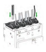
The EverLink lug<sup>9</sup> with creep<sup>10</sup> compensation makes it possible to achieve accurate and durable tightening torque. They minimize loose wiring at installation sites caused by wire strand deformation, terminal temperature changes, and vibration or shocks encountered during equipment transit and handling. EverLink lugs help maintain low-resistance connections for continuity of service.
