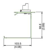
Dimensions 15 to 125 A Circuit Breakers
