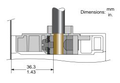
15 to 125 A Circuit Breakers Dimensions
