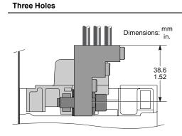
Dimensions 15 to 125 A Circuit Breakers
