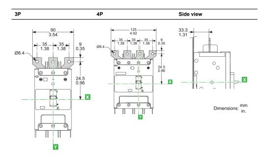
15 to 125 A Circuit Breakers Dimensions
