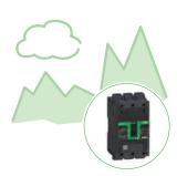
Altitude does not significantly affect the characteristics of PowerPacT B-frame circuit breakers up to 2000 m (6560 ft). Above this altitude, it is necessary to take into account the decrease in the dielectric strength and cooling capacity of air.
