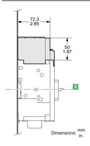
Dimensions 15 to 125 A Circuit Breakers
