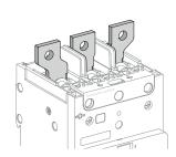
Spreaders can be used to increase the pitch of the circuit breaker from 27 mm (1.063 in.) to 35 mm (1.378 in.). They are delivered with interphase barriers and M8 screws, nuts and washers. The connectors are attached to device terminals equipped with separately provided terminal nut connectors.
