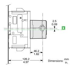
15 to 125 A Circuit Breakers Dimensions
