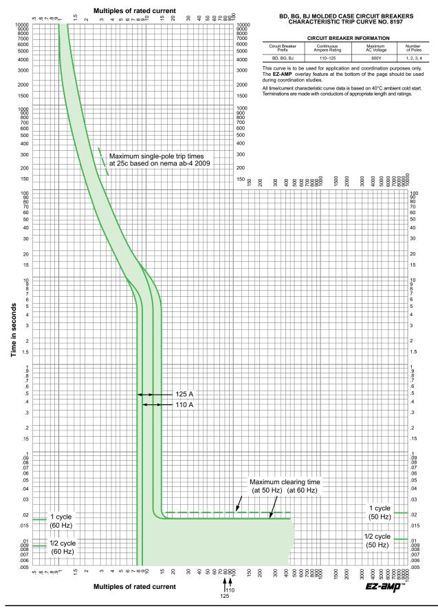
15 to 125 A Circuit Breakers Distribution System
