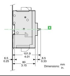
Dimensions 15 to 125 A Circuit Breakers
