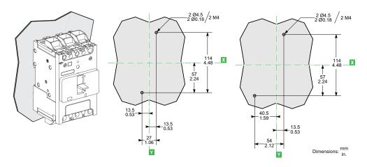
15 to 125 A Circuit Breakers Dimensions
