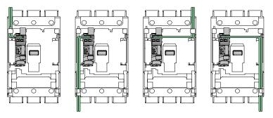
Electrical accessory wire routing can be exited out either of the two load-end corners of the I-Line circuit breaker, under the accessory cover even when using the load-end long terminal shield.
