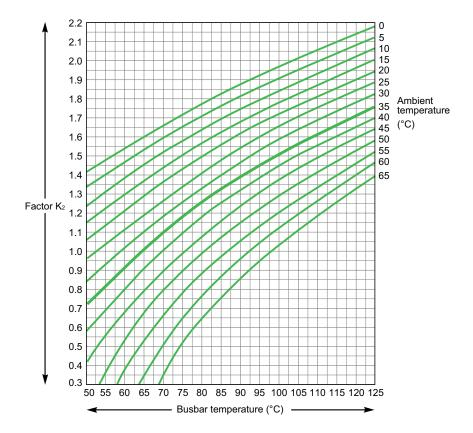
Example: In normal operating conditions, a tinned busbar of 30 x 10 can permanently withstand 630 A.
