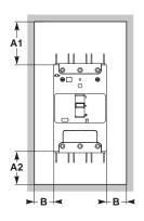
For all types of PowerPacT B-frame circuit breakers that use uninsulated power connections (for example, busbars, spreaders, or uninsulated compression lugs), the minimum clearance distance between the enclosure backplate (grounded metal) and uninsulated power connections is shown below.
