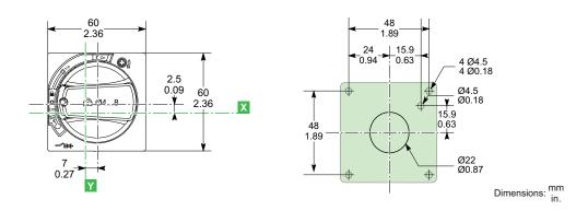
Dimensions 15 to 125 A Circuit Breakers
