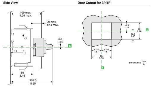
15 to 125 A Circuit Breakers Dimensions
