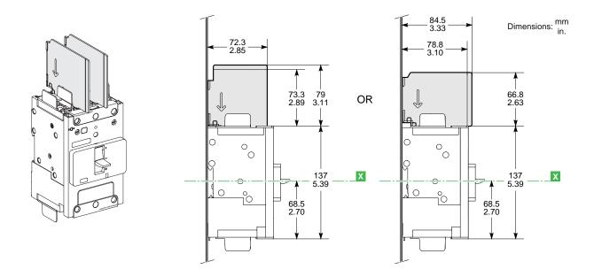
15 to 125 A Circuit Breakers Dimensions
