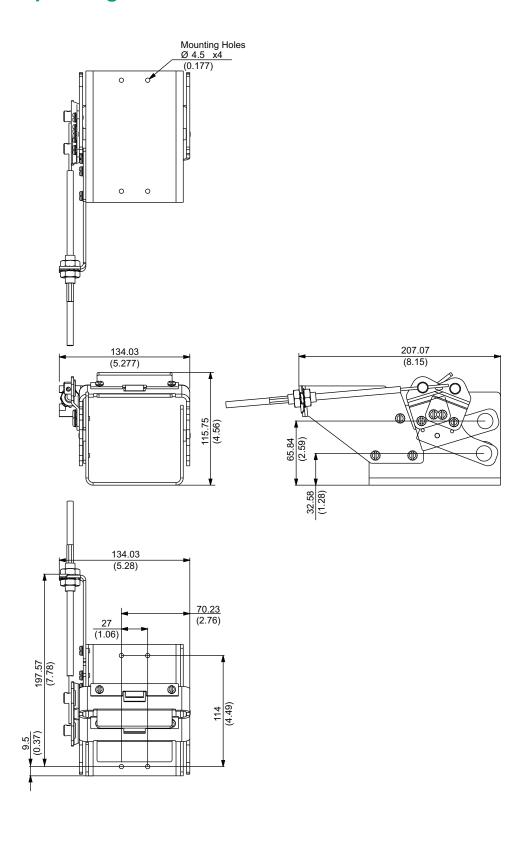
15 to 125 A Circuit Breakers Dimensions
