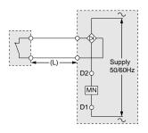
If a longer cable length is required, several solutions are possible to counteract excessive cable capacitance:
